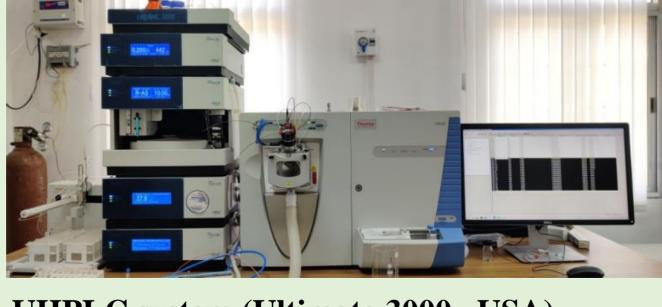
UHPLC system (Ultimate 3000, USA) coupled with a LTQ-XL ion trap mass analyzer
