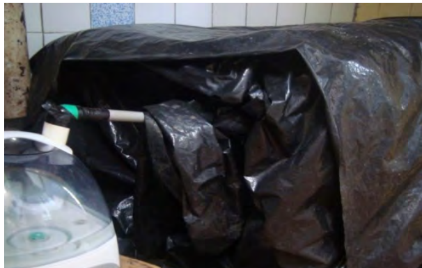
Fig. 14: The dew chamber covered with black polyethylene sheet for about 17 hours.
